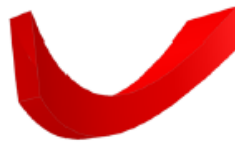
(i) 20-node isoparametric brick
